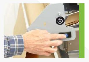
4. Press and release the blue feed button - the paper will load automatically.
