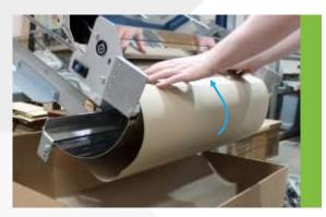
4. Feed the sheet of paper into the entry slot.
