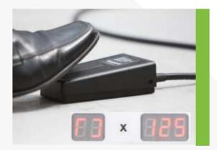
Depress and hold down the footswitch. The length display will increment up as the pack is produced and the quantity display will change to a cycling symbol.
