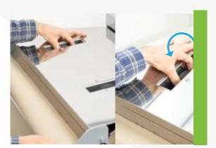
3. Rotate the wheels by hand for about half a turn to feed-in and grip the paper.
