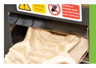
4. The machine will not switch on or start if the outfeed flap is open.
