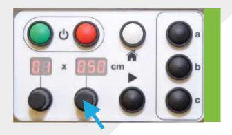
2. Rotate the length knob to the required length.
