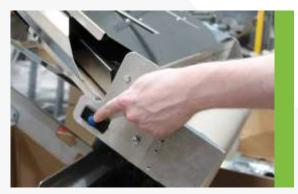
6. Press and release the blue feed button - the paper will load automatically.
