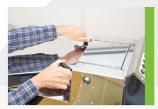
1. Unscrew the two black 'T' handles each side of the top cover until they swing down.
