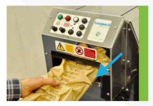
1. Remove any material from the outfeed channel and ensure the outfeed flap is closed.
