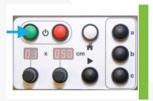
4. Switch the machine on by pressing the green 'I' button. The display will illuminate. If the display shows flashing 'dashes' the machine needs to be loaded with a roll of paper.
