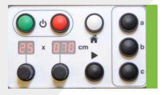
2. Rotate the length knob to the required pack length.
