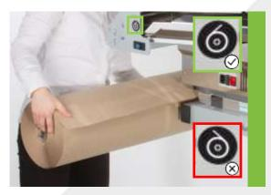
1. Noting the unwind direction, slide a new roll of paper onto the paper arm until the sprung retaining latch springs up.
