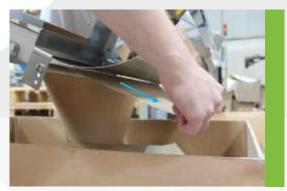
3. Feed the sheet between the guide panel and inner guide rods as shown.
