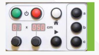
4. Release the preset button to save the values - the display will flash twice before remaining on.
