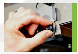
1. Slacken the two black knobs securing the paper off-cuts door under the outfeed channel.
