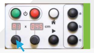
1. Rotate the quantity knob anticlockwise to 'A1'.
