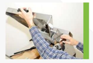
4. Lift the top cover, press the release plunger in and lower the top cover.
