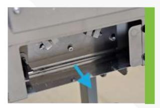
3. Remove any paper off-cuts from around the blade mechanism.
