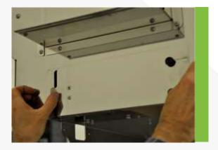
4. Replace the paper off-cuts door taking care to align the safety switch key.
