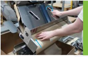
5. Rotate the wheels by hand for about half a turn to feed-in and grip the paper.
