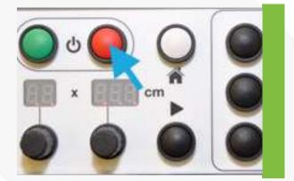
5. Release the preset button to save the values - the display will flash twice before remaining on.
