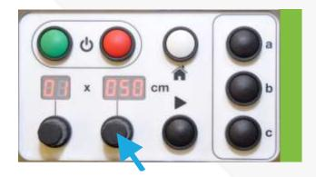
3. Rotate the length knob to the desired length (whilst the display is flashing).
