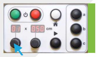
2. Rotate the quantity knob to the desired number from 01 to 99 (whilst the display is flashing).
