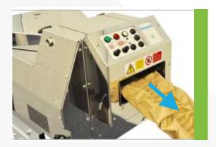
4. Remove the material from the outfeed channel and the machine will generate another pack.
