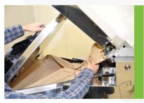
3. Cut the paper across the rods with a knife, at the infeed guide rods.
