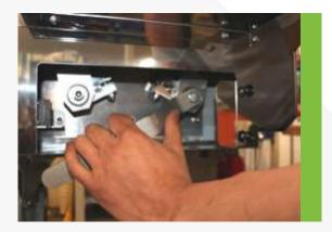
4. Locate the blade reset tool (supplied) on the crank nut.
