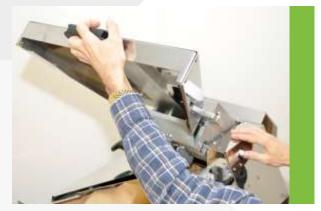
3. The machine will not switch on, or run with the top cover lifted up.
