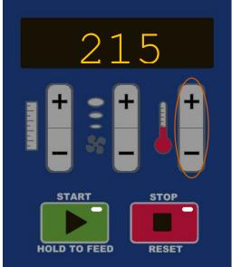
The Temperature Control regulates the temperature of the Seal unit that fuses the front and back film sheets together.
