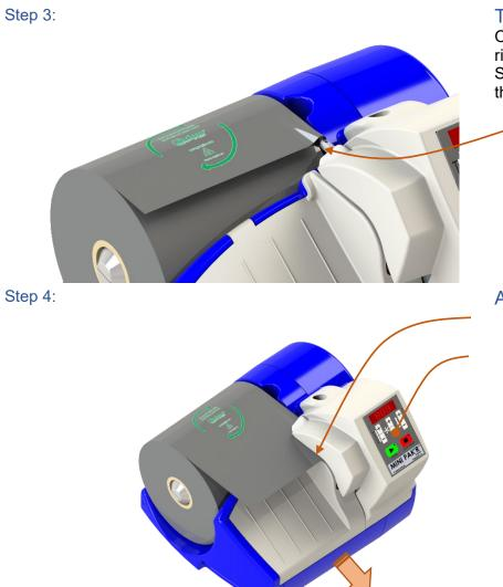
Threading the Film Open the Air Channel at the right side of the Film Roll. Slip the Air Channel over the end of the Air fill tube.
