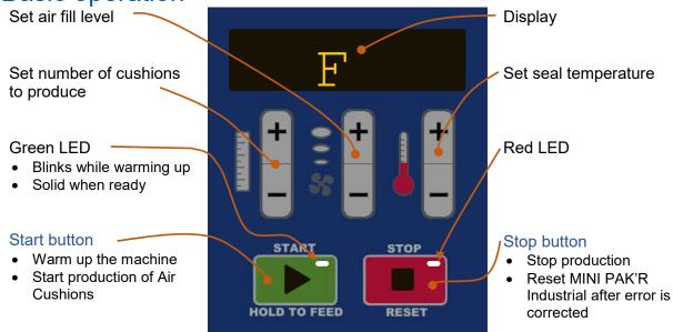
Initially, the display will show "SLP" (Sleep). Once film is loaded, the machine will detect the roll. The green LED on the Start Button will begin flashing. A flashing green LED indicates that the machine is warming to the correct seal temperature. The Control Panel will display seal temperature while adjusting.
