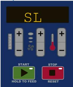
If the machine is not used for 30 minutes, it will enter "Sleep" mode. The Display will read "SLP". To resume Air Cushion production, press the Reset Button. The Seal Bar will begin heating. Press the Start Button again when the green LED remains steady green and the Display reads "rdy" to resume Air Cushion production.
