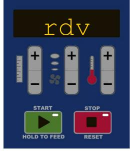
When the green LED remains steady green, and the Display reads "RDY" (Ready), press and release the Start Button again to begin production. The Air Pump will force air into the film, and after a few seconds the Drive Motor will advance the inflated Air Cushions through the Seal Bar and past the Slitting Blade. Air Cushions will emerge at the front of the machine.
